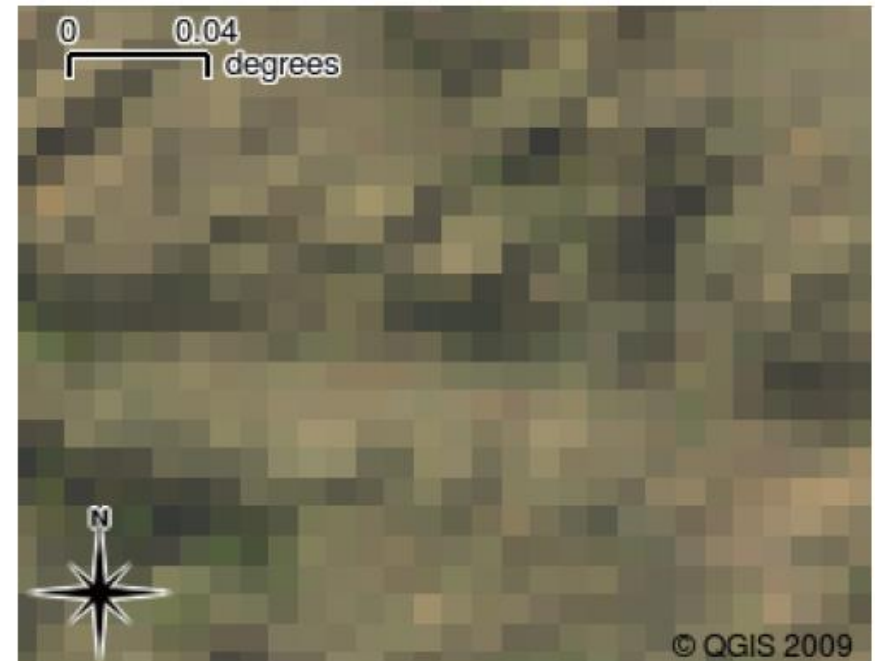
(b) The same raster data, but this time zoomed in. The grid nature of the data can be seen
